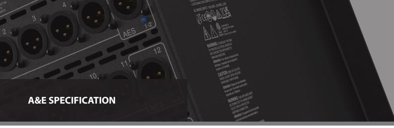
The DiGico DQ-Rack shall have 48 inputs and 20 line outputs. It shall have an additional 4 outputs shall be configurable as either analogue line outputs or AES digtal outputs. The rear panel shall have a Primary and a Secondary EtherCON Dante port. There shall also be a USB Type B port and two redundant PSUs.
